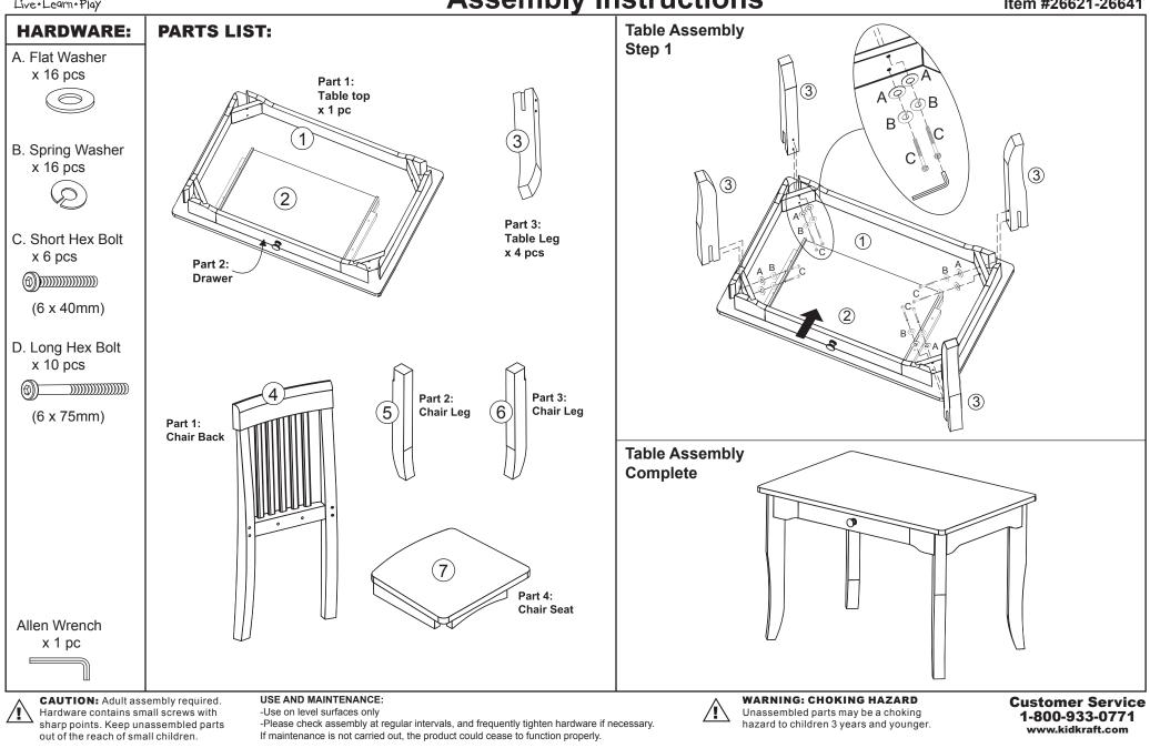
IMPORTANT! DO NOT TIGHTEN SCREWS OR BOLTS UNTIL COMPLETELY ASSEMBLED!!
